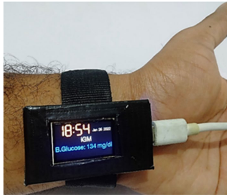
Figure 5. An IoT-enabled real-time blood glucose monitoring system (iGM) deployed in diabetic patient using ESP32 IoT module with organic LED display.
